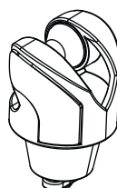
P14 - Roller Assembly (1 pc) NOTE: Attaches to P11 Home Plate
