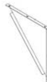
A11 TRIANGLE PANEL - A4M03086 (x4) 13/16"x13 3/4"x13 3/4" (20x350x350)
