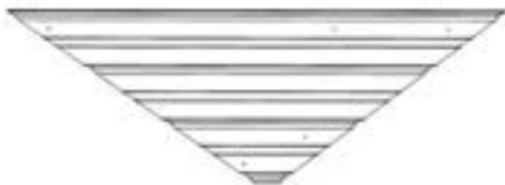
5212 STEEL SHEETING - A4M05212 (x1) 41 11/16"x18 7/8"x1/4" (7x480x1060)
