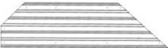
5211 STEEL SHEETING - A4M05211 (x1) 70 1/16"x18 7/8"x1/4" (7x480x1780)
