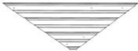
5212 STEEL SHEETING - A4M05212 (x1) 41 11/16"x18 7/8"x1/4" (7x480x1060)
