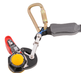
TowerLatch SP with an integral energy absorber ("shock pack") for use where a coil absorber is not present in the vertical lifeline system
