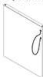
O3 CABINET SIDE PANEL ASSEMBLY M - A4M03077 (x1) 1 3/4"x23 5/16"x26 7/16" (44x592x672)
