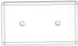
N3 STOP BLOCK - W4L22556 (x1) 5/8"x1 7/8"x3 3/8" (16x48x86)
