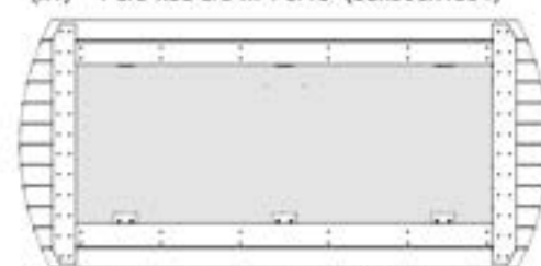
WP04 WALL PANEL ASSEMBLY - W2A04794 (x1) 2 3/8"x35 5/8"x74 9/16" (60x906x201)
