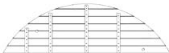
WP01 WALL PANEL ASSEMBLY - W2A04784 (x1) 1 3/8"x19 11/16"x65 3/4" (35x500x1169)
