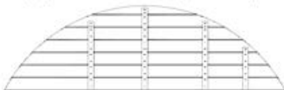
WP03 WALL PANEL ASSEMBLY - W2A04786 (x1) 1 3/8"x20 1/8"x66 1/4" (35x512x1199)
