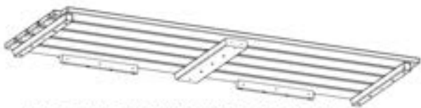
BA02 LEFT BENCH ASSEMBLY - W2A04789 (x1) 19 1/8"57 5/16" (50x486x1456)
