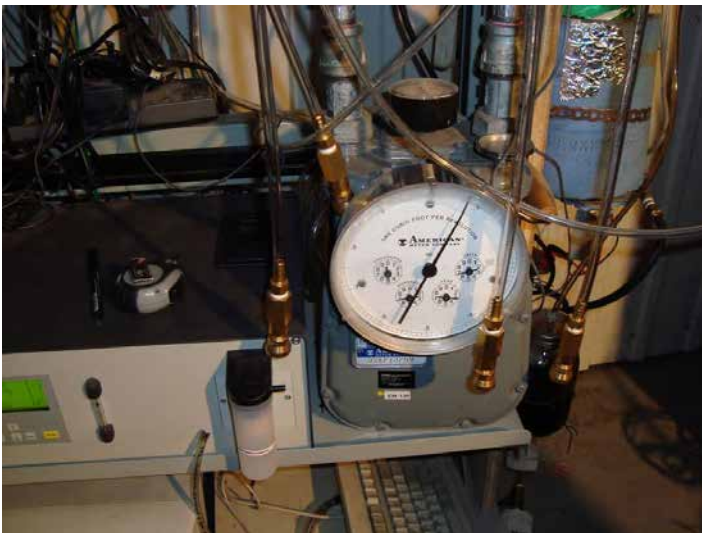
Picture 8 : Reference dry gas meter
