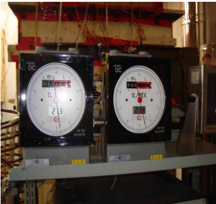
Picture 11: Dry gas meter
