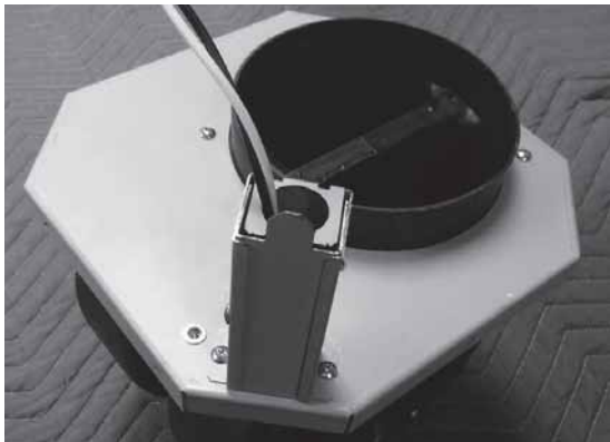
3. Secure AC power wiring box to internal blower flange by (2) M4*8 screws.
