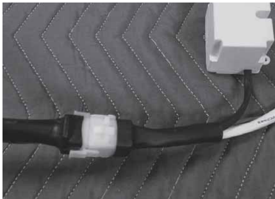
5. Connect 9 pin molex connector from capacitor cable to 9 pin molex connector from internal blower.
