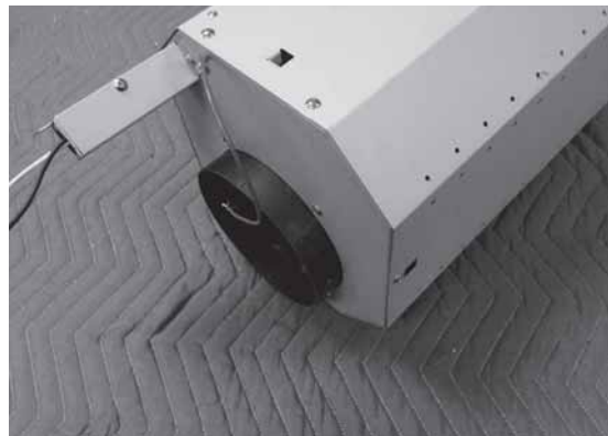
6. Re-install internal blower flange to motor housing by (6) screws previously removed from step 1.
