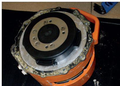
Absorber Cover Plate Removed
