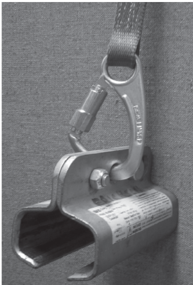
Figure 6 Carabiner connected through the closed eye of the Rail Slider
