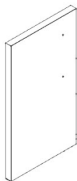
D5 PIZZA OVEN CABINET DOOR ASSEMBLY L - A4M03087 (x1) 1 5/16"x15 9/16"x28 1/8" (34x396x715)
