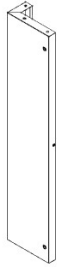
G8 RIGHT CORNER CABINET SIDE WALL ASSEMBLY M - A4M03042 (x1) 3 1/8"x7 1/16"x33 3/8" (80x180x848)
