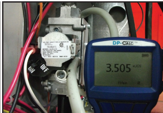
FIG. 30. - MANOMETER MEASURING GAS MANIFOLD PRESSURE
