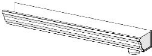
FRONT RIGHT GUTTER W/ OUTLET - STEP 2
