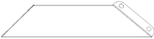
D05 CORBEL - A4M01831 (x1) 2 3/4"x5 7/8"x24 13/16" (70x149x631)
