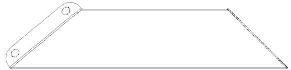
D06 CORBEL - A4M01832 (x1) 2 3/4"x5 7/8"x24 13/16" (70x149x631)
