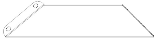
D06 CORBEL - A4M01832 (x1) 2 3/4"x5 7/8"x24 13/16" (70x149x631)
