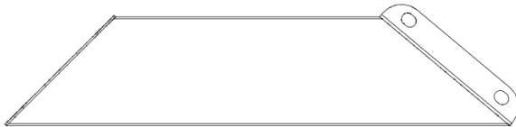
D05 CORBEL - A4M01831 (x1) 2 3/4"x5 7/8"x24 13/16" (70x149x631)
