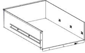
D4 CABINET DRAWER BODY ASSEMBLY - A4M03571 (x2) 22 1/4"x16 1/16"x6 7/16" (164x408x565)
