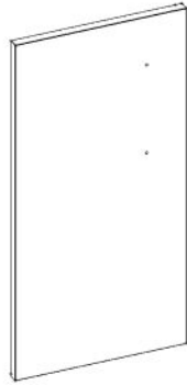
D23 CABINET FRONT DOOR ASSEMBLY - A4M04720 (x1) 33 1/16"x16 1/16"x15/16" (24x408x840)
