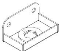
A9 HOSE BRACKET ASSEMBLY - A4M03060 (x1) 1 1/4"x1 7/16"x2 9/16" (31x36x65)
