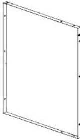
G14 CABINET BACK PANEL ASSEMBLY - A4M04716 (x1) 27 5/16"x33 3/8"x1 3/16" (30x847x693)
