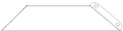
D05 CORBEL - A4M01831 (x1) 2 3/4"x5 7/8"x24 13/16" (70x149x631)
