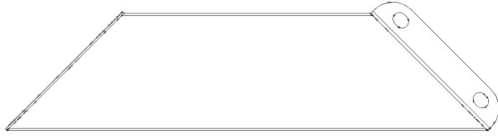
D01 CORBEL - A4M01817 (x1) 2 3/4"x5 13/16"x22 1/4" (70x147x565)
