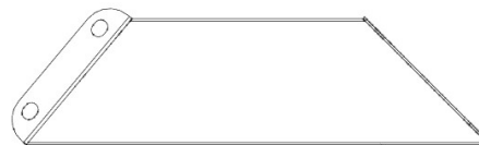
D03 CORBEL - A4M01826 (x1) 2 3/4"x5 11/16"x20 1/16" (70x145x509)
