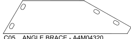
C05 ANGLE BRACE - A4M04320 (x2) 1 7/16"x5 5/16"x20 1/16" (36x135x509)
