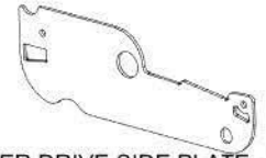
L02 LOUVER DRIVE SIDE PLATE - A4M04139 (x1) 1/16"x2 3/16"x6 9/16" (2x55x167)
