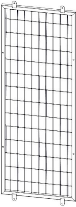
MP01 METAL PANEL - A4M02614 (x5) 1 1/16"X20 1/2"X58 9/16" (27.4x520x1488)
