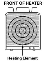
**NOTE:** During the heaters initial use, you may experience a slight odor or smoking. This is the result of the heating element fabrication protective coating "burning off". This is normal and will go away after a few minutes of use.
