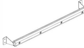
H01 DOOR HANDLE ASSEMBLY - A4M02761 (x1) 2 3/8"x3 3/4"x30 1/4" (60x95x769)
