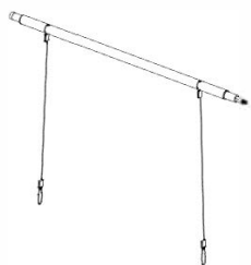
S01 SPINDLE ASSEMBLY - A4M02150 (x1) 1 3/16"x37 5/8" (x30x955)
