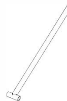
R04 PIVOT ROD - A4M02784 (x1) 1/2"x1 7/16"x12 1/4" (12x36x312)
