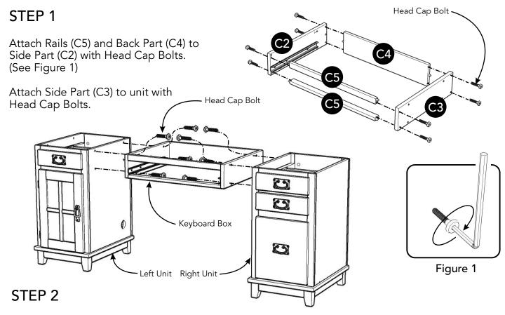
Attach Left Unit and Right Unit to Keyboard Box with Head Cap Bolts.
