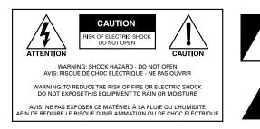
The lightning flash with arrowhead symbol within an equilateral triangle, is intended to alert the user to the presence of uninsulated "dangerous voltage " within the product's enclosure that may be of sufficient magnitude to constitute a risk of electric shock to persons.
