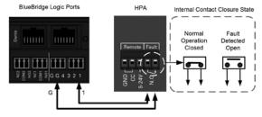
This example shows the HPA Remote Fault connected to a BlueBridge<sup>®</sup> Logic port to create an AMP Status Indicator on a Touchscreen.
