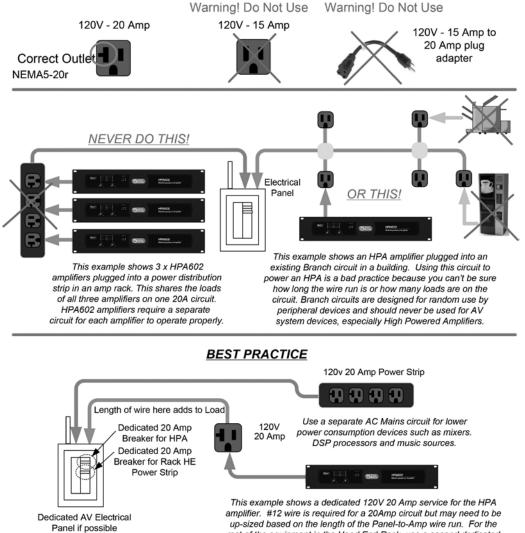
rest of the equipment in the Head End Rack, use a second dedicated 20 amp circuit to the power Strip.
