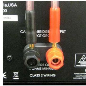
Inserting banana plugs into wire holes
