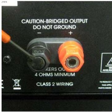
Removing the binding post insulators
