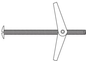
**Toggle Bolt** - Drill hole through wall. Hole must be large enough for the wings to pass through. Insert screw through the holes in the dartboard and thread the toggle wings just onto the screw. Fold the wings back and push through the hole until the wings spring open. Pull back on the screw to hold wings against the inside of the wall and tighten screw.
