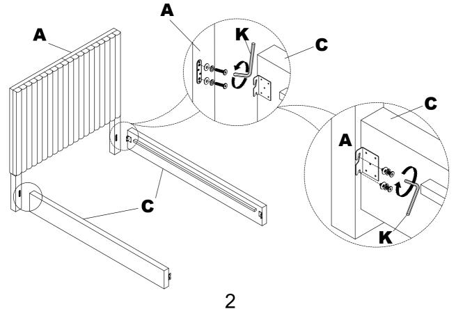
3 Unfasten the Bolts, Spring Washers and Flat Washers on Footboard (B), then attach Side Rail (C) to Footboard (B) using all of these hardware and tighten with Allen Key (K). Remark: Do not tighten the bolts until screw Slat Roll (E) well on the Side Rail (C).
