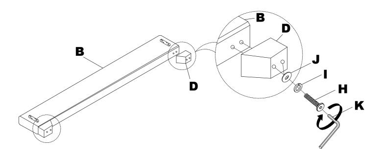
2 Unfasten the Bolts, Spring Washers and Flat Washers on Left & Right Leg of Headboard (A), then attach Side Rail (C) to Headboard (A) using all of these hardware and tighten with Allen Key (K). Remark: Do not tighten the bolts until screw Slat Roll (E) well on the Side Rail (C).
