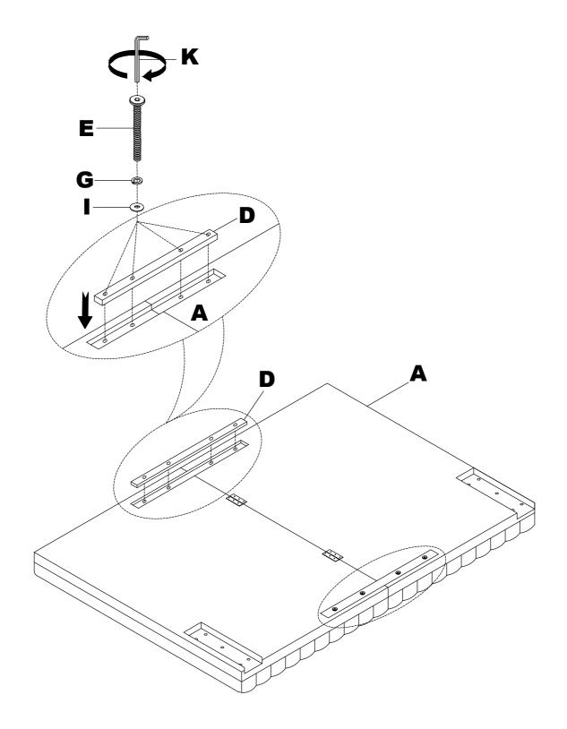
4 Attach Left & Right Leg (B&C) to Headboard (A) by using Allen Bolt (E), Spring Washer (G) and Flat Washer (I) and tightening with Allen Key (K).
