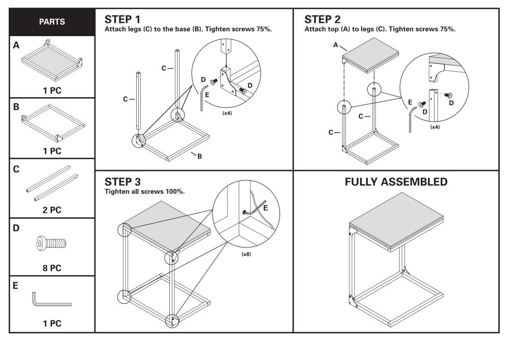
NOTE: 25 LB. WEIGHT LIMIT. FEET ON BOTTOM (B) ARE ADJUSTABLE FOR LEVELING.
