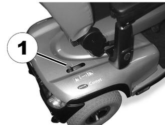
The lever for engaging and disengaging the motor is located on the right-hand side at the rear.
