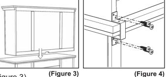
Attach Steel Plate Connectors on the back of the units by inserting Wood Screws and tighten. (See Figure 4)
