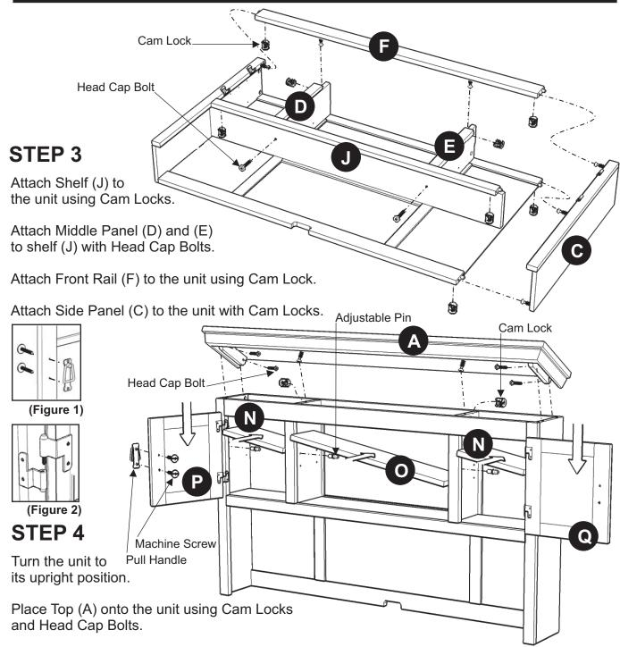
Insert Adjustable Pins into side panels and middle panels at the desired level
