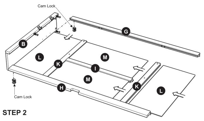
Attach Back Stretcher (H) to Side Panel (B) using Cam Lock.
