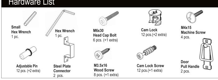
Tools required for assembly: Phillips screwdriver
