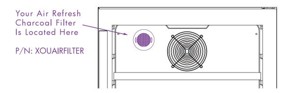
Rotate the filter 1/4 turn to unlock
