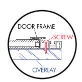
7 Using the (10) ST4-30 self-tapping screws supplied securely fasten the frame to the door. Do not over tighten as screws may strip out. WARNING: Screws are sized for 3/4" panel, DO NOT USE these screws for thinner panels.
