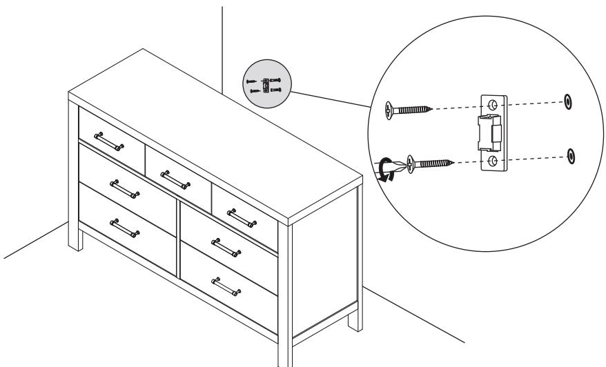
Loop provided 2 ties through both brackets and secure tightly.
