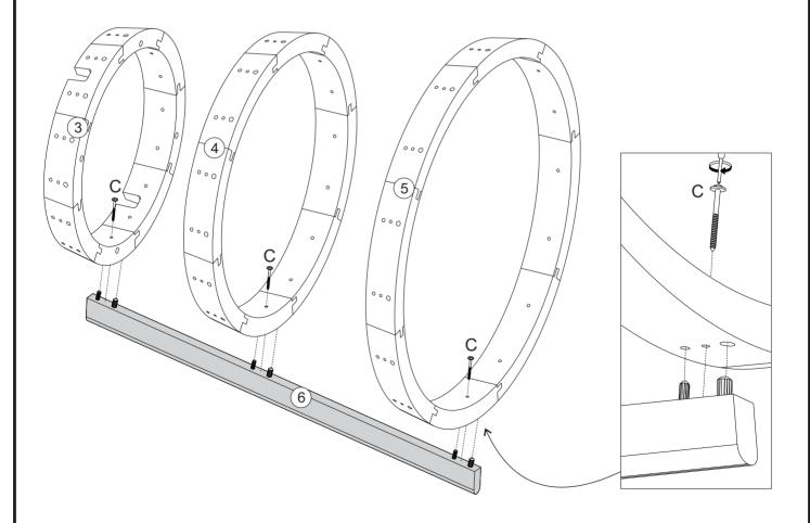
Fix one vertical rail 6 on the assembled bases 3, 4 and 5 with the screws (C),using Phillips Head Screwdriver.
