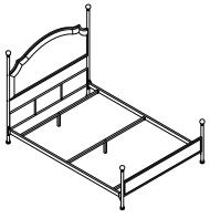
Assemble the left lower posts (A) and the right lower posts (B) to the headboard panel (F) with 4pcs Bolt (L) then fastened using allen wrench (U).
