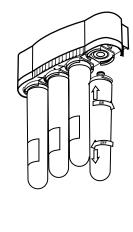
Remove the red SFC tubing from the fitting before completely removing the RO membrane module
