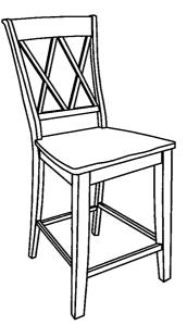
Stand chair up on an even surface and check that it is balanced. If there is a slight wobble, apply downward pressure in the corner where a leg is uneven. Keeping pressure in that corner, tighten all bolts. If balanced, apply downward pressure evenly in the center and tighten all bolts. Do not over-tighten beyond hole depth.
