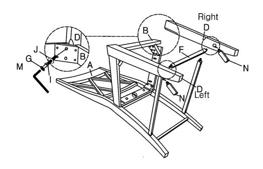
4 Insert Pan Head Screw (L) into the holes of Front Leg (D) and Stretcher (F) by using Screwdriver (not included).
