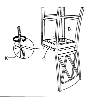
Turn the assembled chair to the upright position carefully. Make sure the chair is level, and then securely tighten all bolts at this stage. Assembly is now completed.
