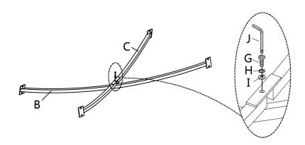
Attach Lower Connecting Rod (B) and Upper Connecting Rod (C) to Leg (E) using Bolt (G), Spring Washer (H), Flat Washer (I) with Allen Key (J).
