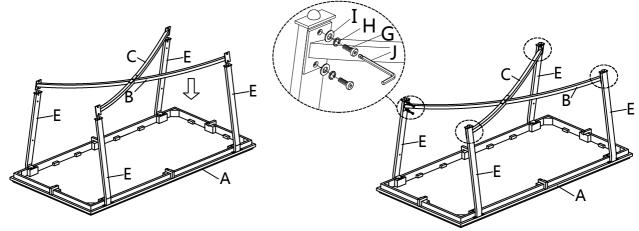
Use Long Bolt (F), Spring Washer (H), Flat Washer (I) with Allen Key (J) to fix Leg (E) and Table Top (A).
