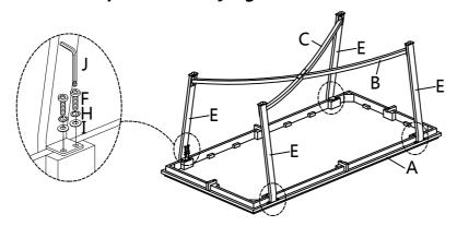
Attach Rail (D) to Leg (E) and Table Top (A) using Bolt (G), Spring Washer (H), Flat Washer (I) with Allen Key (J).
