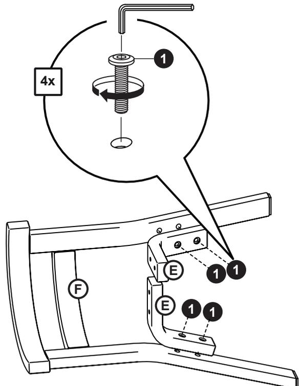
**3** Ensure that each set screw is fully tightened upon completion of assembly. Do not overtighten.
