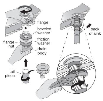
\* Note: Attach tail piece to drain body using teflon tape. tape or plumber's putty.
