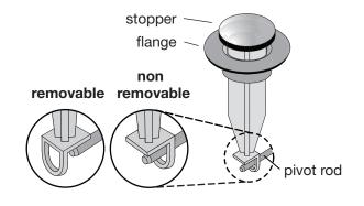
Step 6 Attach pivot rod to drain body
