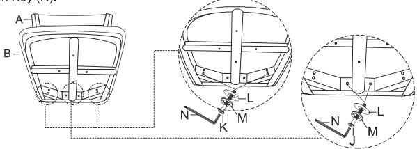
Keep the Backrest (A) and Cushion Seat (B) inverting on a stable raised surface. Attach the Swivel Plate located on the Apron with Swivel Plate (E) to the Cushion Seat (B) using JCBC Screw (I), Flat Washer (L) with Allen Key (N). Turn the Chair right side up.
