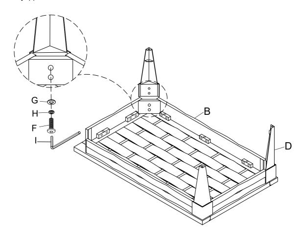
First, assemble Bottom Panel (C) to Leg (D), using Bolt (E), Lock Washer (H) and Flat Washer (G) by Allen Key (I). Second, assemble the last Leg (D) to Top Frame (B) & Bottom Panel (C), using Bolt (F), Bolt (E), Lock Washer (H) and Flat Washer (G) by Allen
