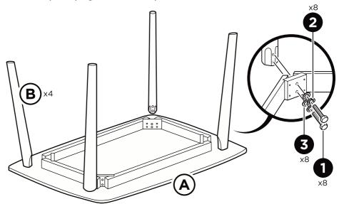
Repeat to attach the remaining table legs, then place one **part 4 foot pad** on the bottom of each leg. Flip the assembled table upright.
