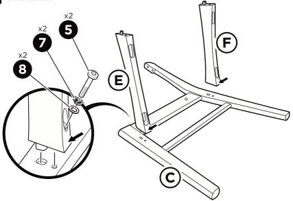
Attach one part D left chair frame onto the chair assembly, then secure the part E & F supports with two part 5 bolts, two part 7 spring washers, and two part 8 flat washers.
