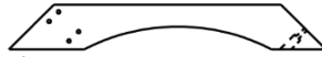
D11 | CALE ANGULAIRE LONGUE - W4L13482 (x3) | 1 3/8 po x 5 1/4 po x 37 1/8 po (36 x 134 x 942)
