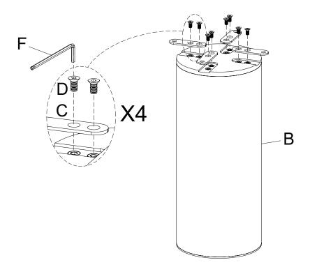
Attach the Column Base (B) to the Top Panel (A) using Bolt (E) through the Metal Bracket (C) with the Allen Key (F).
