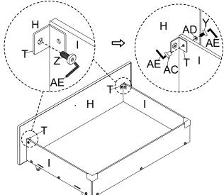
Insert the Bolt (AA) and Washer (AD) to the back of Drawer Front Board (H), turn the L-Allen Key (AE) to tighten them.
