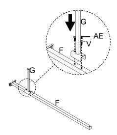
Attach the Center Rail - Front / Rear (F) to the Headboard (A) and the Footboard (B), insert the Bolt (V), turn the L-Allen Key (AE) to tighten them. Then attach the Center Rail - Front / Rear (F) to the Center Support Bar (C), insert the Bolt (W), turn the L-Allen Key (AE) to tighten them.
