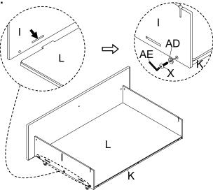
Attach the Drawer Back Board (J) to the Drawer Bottom Frame (K), insert the Bolt (X) and Washer (AD), turn the L-Allen Key (AE) to tighten them. Attach the Drawer Board Connector (Q) to the assembled drawer, insert them into correct places.
