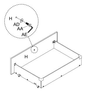
Align drawers with the bed frame and push them into the bed. Lock drawers by slightly lifting drawers and insert the Pin that the head of Bolt (AA) into the Slot.
