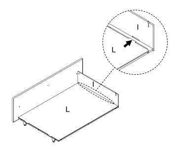
Insert another Drawer Side Board (I) to the Drawer Bottom Board (L) first, and attach the Drawer Side Board (I) to the Drawer Bottom Frame (K), then insert the Bolt (X) and Washer (AD), turn the L-Allen Key (AE) to tighten them.
