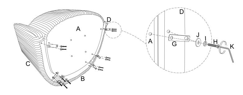
4 Attach the Swivel Base (E) to the Cushion Seat (A) using Bolt (H), Spring Washer (I) and Flat Washer (J) with the Allen Key (K). First, secure two holes, then rotate and secure the other two
