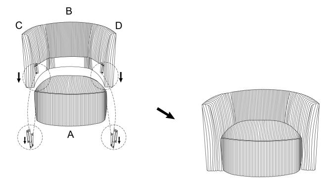
Attach the Backrest (C & B & D) to the Cushion Seat (A) by the Metal Connector (G) using Bolt (H), Spring Washer (I) and Flat Washer (J) with the Allen Key (K).
