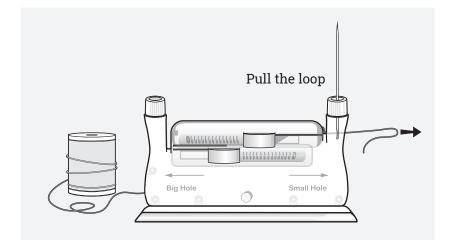
6. Lift the threaded needle from funnel; cut thread to desired length.
