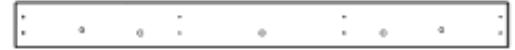
AD01 SUPPORT DE FAÎTE - W4L21900 (x1) 15/16 po x 4 po x 43 7/16 po (24x102x1103)
