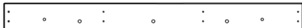
AD01 SUPPORT DE FAÎTE - W4L21900 (x2) 15/16 po x 4 po x 43 7/16 po (24x102x1103)
