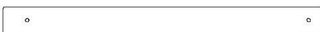
J7 | PLANCHE INFÉRIEURE - W4L12471 (x1) | 1 po x 2-3/8 po x 28-3/8 po (24 x 60 x 720)
