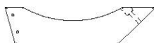
H10 | CALE ANGULAIRE - W4L12460 (x4) | 1 po x 3-3/8 po x 13-3/8 po (24 x 86 x 340)
