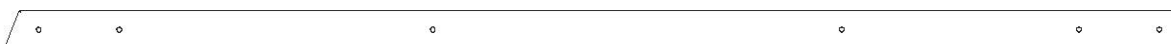
F4 | PLANCHE DE SOL - W4L12487 (x1) 1-3/8 po x 2-3/8 po x 74-1/8 po (36 x 60 x 1883)
