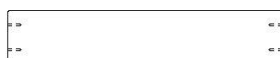
H5 | SOLIVE DE PLANCHER - W4L12455 (x1) | 1 po x 3-3/8 po x 17-1/4 po (24 x 86 x 438)
