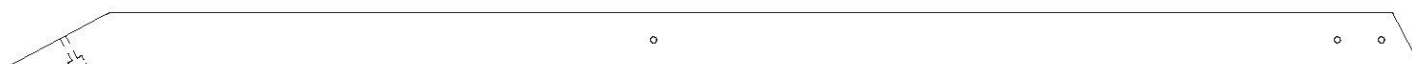
E2 | CALE ANGULAIRE - W4L12328 (x2) 1-3/8 po x 3-3/8 po x 88-3/4 po (36 x 86 x 2254)
