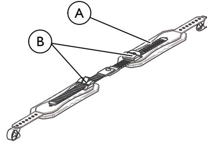
Attach click strap **A** with web mount to the seat or back frame as shown in photo below.
