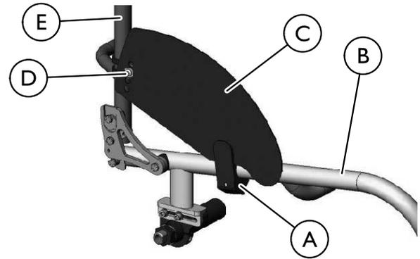
**i** If sideguard will not pivot freely, bolt through sideguard clamp (D) and sideguard (C) is too tight. To correct, loosen bolt.
