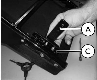
I. Attach the L Brackets (A) to the inside of the welded tabs (C) on the seat frame by:
