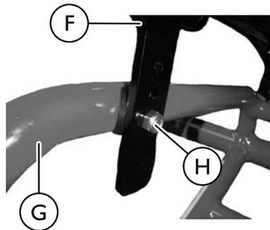
5. Place a flat and coped washer on each bolt, and insert the bolts through the drilled holes in the front of the seat frame (D).
