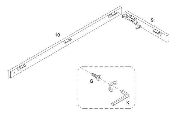
Using bolt (G) attach connecting iron sheet on part (9) to part (10) with Hex key (K) as per diagram.
