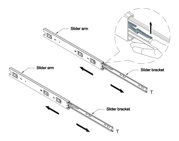
Pick up the slider arm (T) and separate the slide runner for the following Steps. Extend the slide runner all the way forward, press the plastic release lever of the slider arm up and pull the slide runner complete out .
