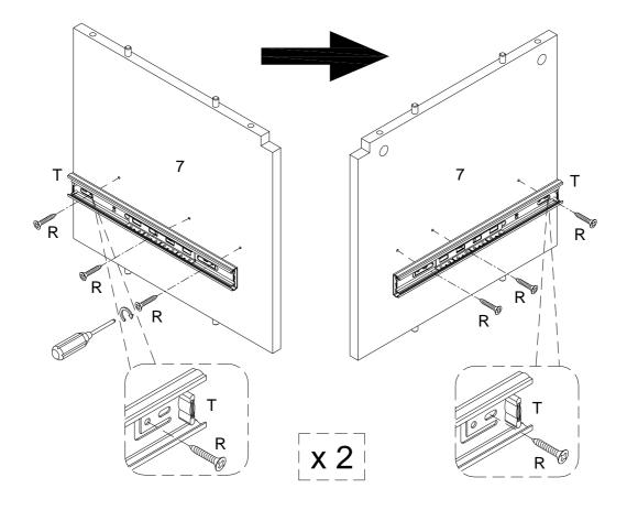
Using screw (R) attach Drawer slider (T) to part (7) with Philips head screwdriver as per diagram.
