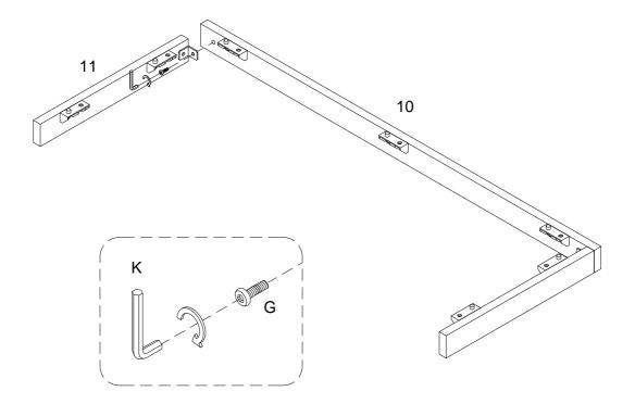
Using bolt (G) attach connecting iron sheet on part (11) to part (10) with Hex key (K) as per diagram.
