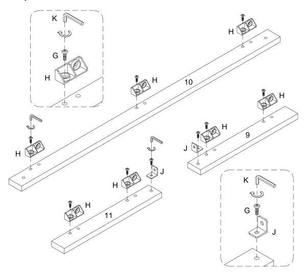
Using Bolt (G) attach plastic wedge (H) to parts (9,10,11) ,and using bolt (G) attach Connecting iron sheet (J) to parts (9,11) with Hex key (K) as per diagram.
