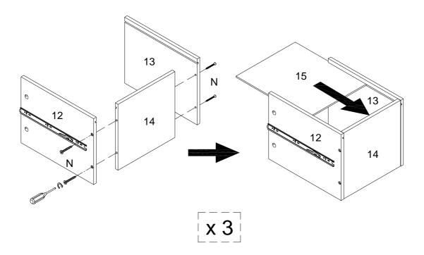
Using screw (N) attach parts (12,13) to part (14) with Philips head screwdriver, then put part (15) as per diagram.
