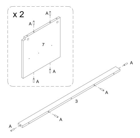
Insert wooden dowel (A) into parts (3,7) as per diagram.
