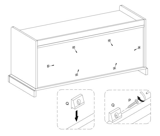
Using screw (P) secure plastic wedge (Q) with Philips head screwdriver as per diagram.
