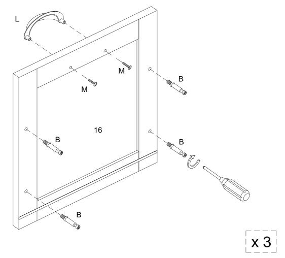
Secure cam bolt (B) into part (16), and using handle bolt (M) secure handle (L) to part (16) with Philips head screwdriver as per diagram.
