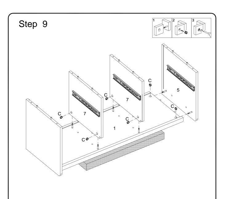
Using Cam lock(C) secure parts (5,7) to part (1) with Philips head screwdriver as per diagram.
