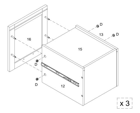
Using Cam lock(D) secure part (16) to parts (12,13) with Philips head screwdriver as per diagram.
