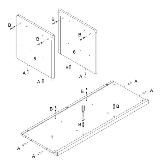
Insert wooden dowel (A) into parts (1,5,6), then secure cam bolt (B) into parts (1,5,6) with Philips head screwdriver as per diagram.
