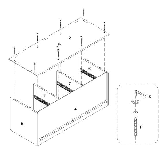
Using screw (F) attach part (2) into parts (5,6,7) with Hex key (K) as per diagram.
