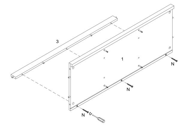
Using screw (N) secure part (3) to part (1) with Philips head screwdriver as per diagram.
