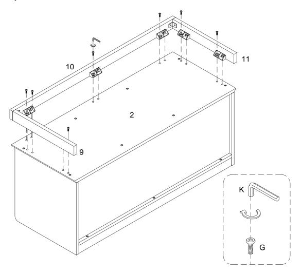
Using bolt (G) attach plastic wedge on parts (9,10,11) to part (2) with Hex key (K) as per diagram.
