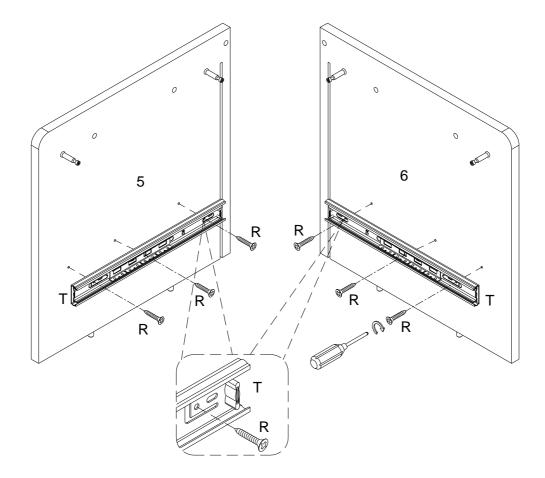
Using screw (R) attach Drawer slider (T) to parts (5,6) with Philips head screwdriver as per diagram.
